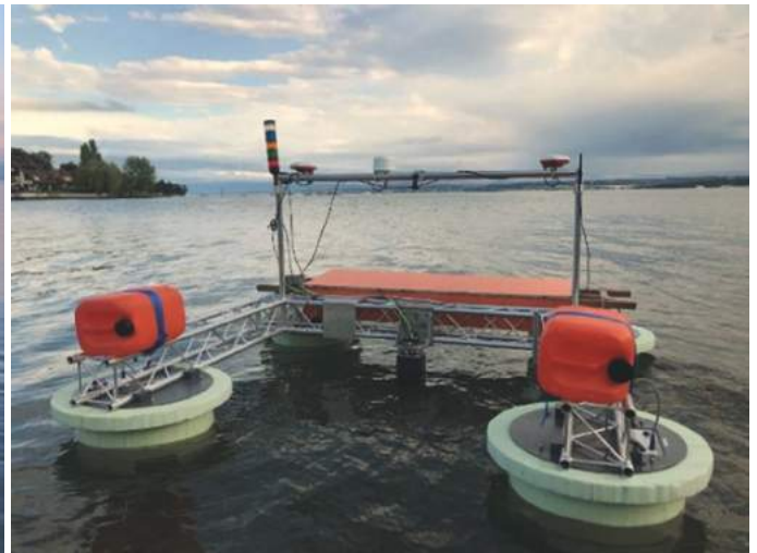
HydroCrawler Generation 1 (links) und Generation 2 (rechts) bei Messfahrten auf dem Bodensee HydroCrawler generation 1 (left) and generation 2 (right) during measuring runs on Lake Constance
