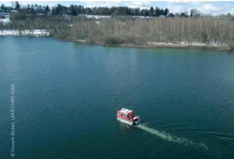
Acquisition bathymétrique à proximité de la rive occidentale du lac de Chalain. Bathymetric acquisition near the western shore of Lake Chalain.
