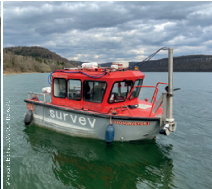
Le Geosurveyor I (GEOxyz) et son équipement sonar avant immersion. The Geosurveyor I (GEOxyz) and its sonar equipment before immersion.
